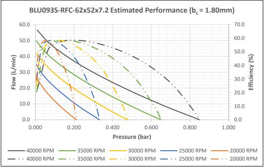
Increasing channel depth to 1.80mm allows for an estimated increase in flow of approximately 32% while still delivering an estimated output pressure of more than 2x that of the original 47mm design. Note how the performance curve has shifted, allowing for increased flow with decreased pressure by simply changing the depth of the side channel while utilizing the same impeller.
