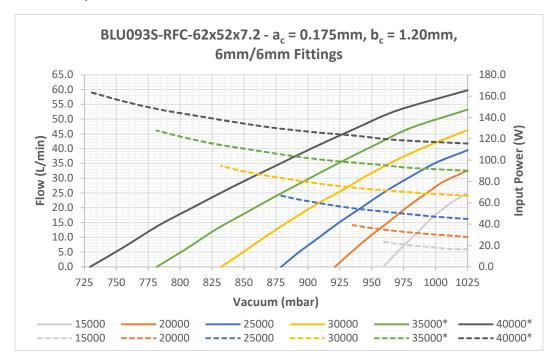
Vacuum performance followed the same trend as pressure performance with measured improvements only possible with increased input power. Unlike the pressure curve, the vacuum curves didn't flatten out as much with the 0.175mm axial clearance compared to the 0.200mm clearance.
