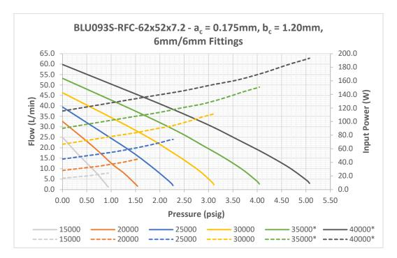
Free flow and maximum pressure increased at each speed but not without corresponding increase in input power, providing a negligible efficiency improvement by reducing the axial clearance at this point. The shape of the curves did flatten out somewhat with a concave shape not seen until the compressor is closer to maximum pressure and low flow.
