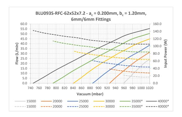
Vacuum performance closely tracked pressure performance in terms of characteristic curve shape with the main difference being lower input power required at maximum vacuum per speed compared to maximum pressure. This is the same trend that was seen when testing the 3D printed plastic prototypes in 2020. Once again, 35,000 and 40,000 RPM were extrapolated from the lower speeds where the motor was able to run without overheating.
