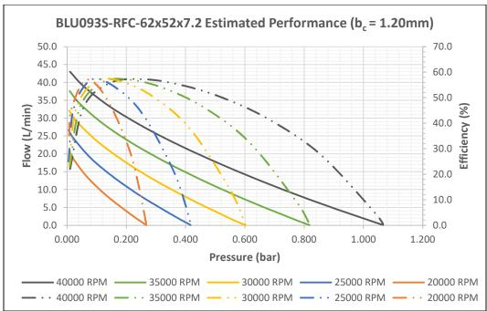
An impeller diameter of 62mm versus the original 47mm allows for an estimated increase in flow and pressure at the same compressor speeds when combined with a  $b_c$  = 1.20mm channel depth. The output pressure estimate is approximately 3x that of the original 47mm design.
