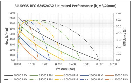
Increasing channel depth even further to 3.20mm we see that the flow estimate is now approximately double the original 47mm design. Maximum output pressure has dropped significantly compared to the 62mm impeller with the 1.20mm side channel depth, but the overall compressor performance envelope is still significantly broader than the originally proposed design.
