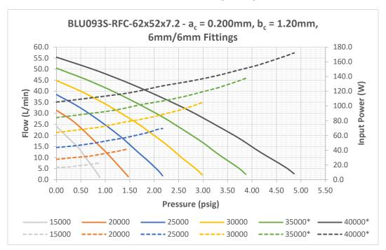
What is immediately apparent from the above pressure curve is how low the output pressures are and how high the input power requirements are compared to the estimated values. Granted, input power shown is the RMS power of the whole system calculated by multiplying input current by input voltage and not just of the compressor end, but these values are still significantly higher than expected.
