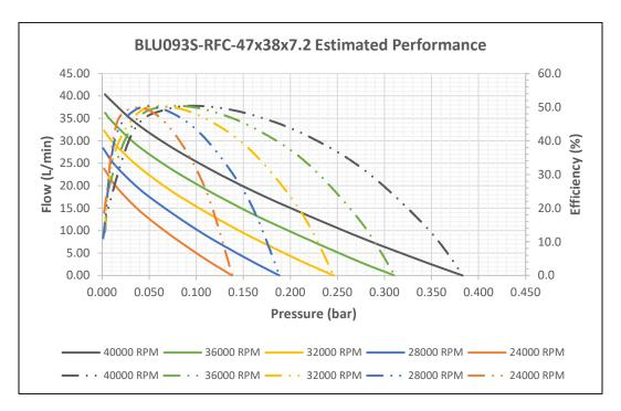
Looking at the required power of the compressor plus the impeller flywheel power (the power required just to spin the impeller at speed – see Appendix A) it was felt the compressor was undersized for the selected 84W motor and a slightly larger compressor could be developed. The decision to increase the size of the compressor was made based on the assumption that the Excel calculations were correct and that the 84W motor was rated at its nominal, 24VDC speed of 34,400 RPM.
