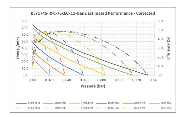
The updated efficiency curve has changed notably with predicted maximum efficiency of 48% versus the original predicted efficiency of 72%. Based on the data available in past and current literature, maximum efficiency for regenerative flow compressors is typically 50% or less, so the updated efficiency curve helps boost confidence in this portion of the mathematical model.
