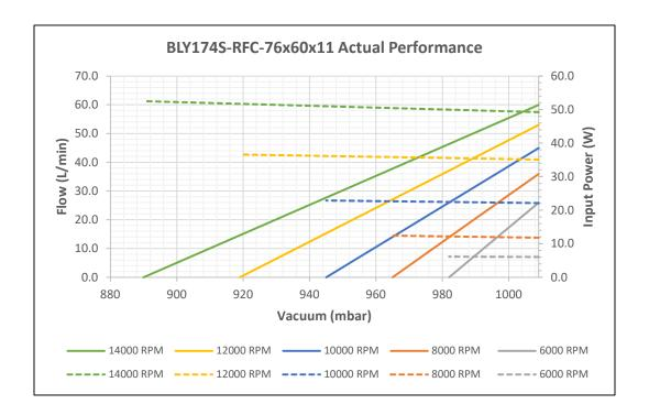
The above BLY174S-RFC curves and those that follow for the Gen2 iteration show input power with approximate motor and controller losses subtracted to clarify the power consumption of just the compressor end. The efficiency curve for the motor, as provided by Anaheim Automation, along with the calculated electrical power losses used can be found in Appendix B.
