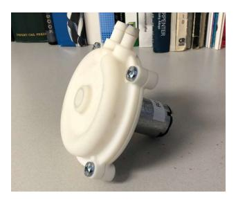
While the name of this configuration is G30-RFC-76x60x11, the actual impeller width was machined down to 10.85 mm to allow for axial clearance in the volute, and as such the impeller channel depth was reduced to approximately 4.83 mm. For clarification on the remaining curves, flow vs. pressure is shown as solid lines while power vs. pressure and efficiency vs. pressure are shown as dashed lines.
