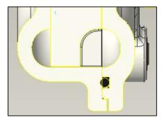
It was theorized that these two profiles cannot be mixed, or the pressure developed in the impeller will dissipate almost immediately as it crashes into the outer wall of the tightly fitted volute. The air does not have the space to follow the helical trajectory created by the RFC unless the impeller and volute/head profiles are matched as shown below.
