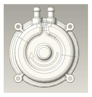
A second low-cost experiment is to develop a pneumatic set that uses semi-circular impeller blade profiles. This design theoretically reduces the tendency of the air to crash into any sharp corners inside the compressor by forcing the air to move in a circular pattern versus an elliptical pattern, and according to the limited literature improves overall efficiency. It is unknown how well the Excel model can predict
