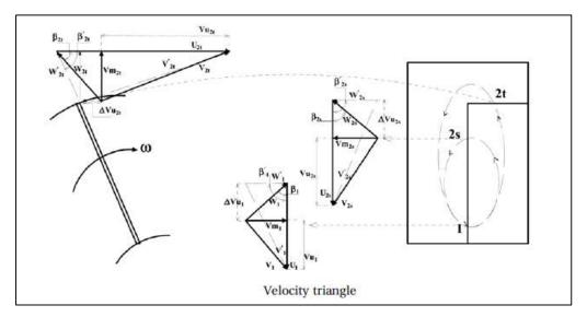
To render the velocities more realistic, slip factors need to be considered. For the blade side this factor can be calculated as
