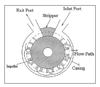
The compressor housing contains a "stripper" that separates the inlet and outlet ports of the compressor. The clearances between the impeller and compressor housing, and more specifically the stripper, are minimized to reduce leakage flow and improve overall system efficiency.
