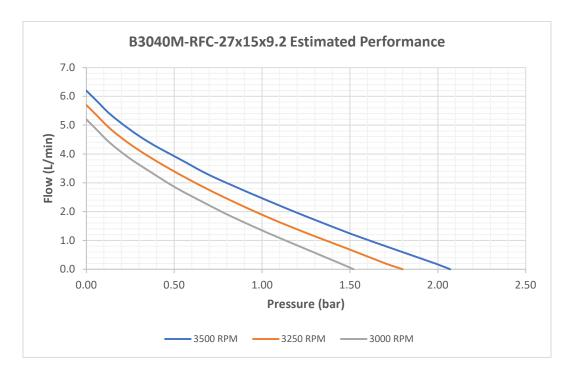
The B3040M-RFC-27x15x9.2 configuration was designed as the Excel calculator was still under development and additional knowledge was still being gathered on the performance characteristics of the RFC. There was a unit conversion error discovered after initial testing that proved this optimistic performance to be unrealistic.
