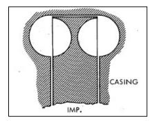
It is worth pointing out that while far less research and testing have been performed on semi-circular blade profiles compared to straight radial blades, it has been proven that total pump output pressure and efficiency are increased with semi-circular blades.
